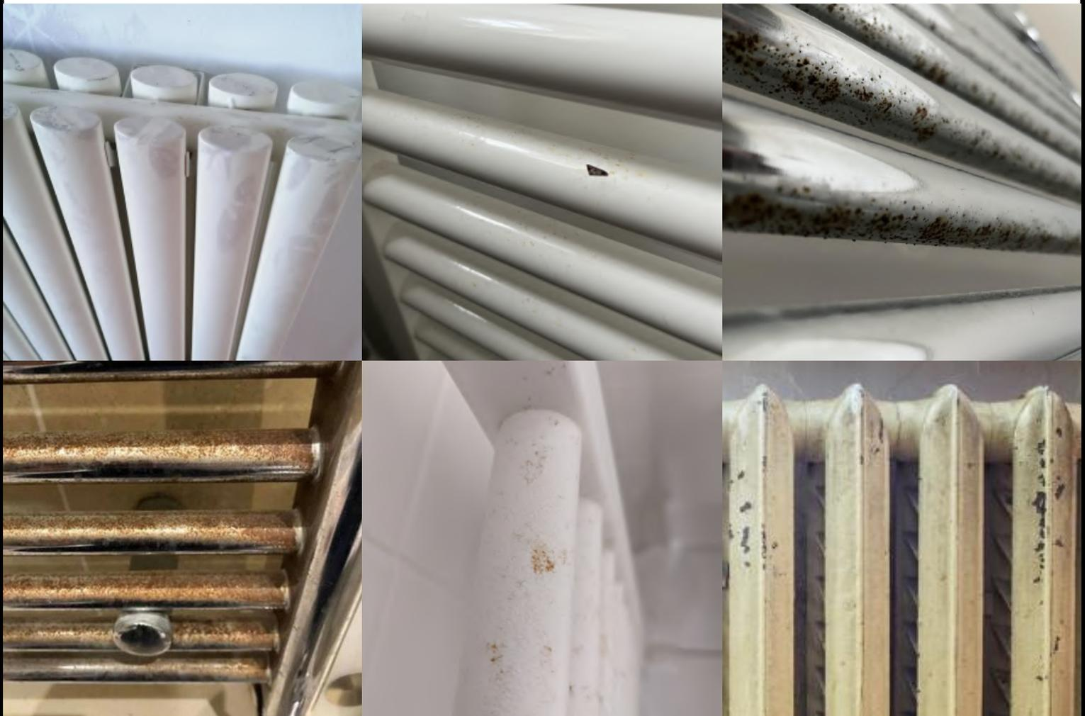
The images above show issues such as rusting, peeling, discoloration, and tarnishing, all resulting from improper cleaning of radiators and towel rails.
